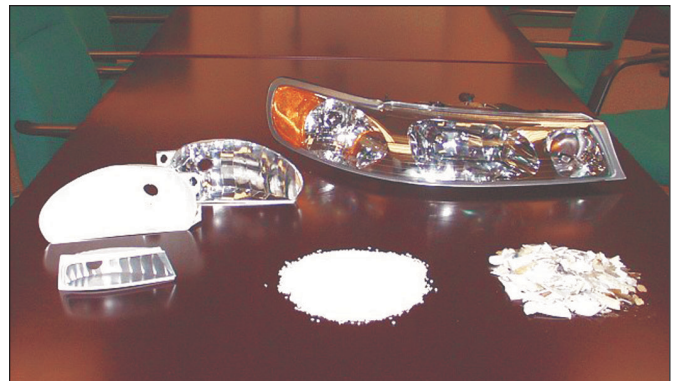
Materials recovered from ELVs can be used to manufacture new vehicle parts and other plastic products.
